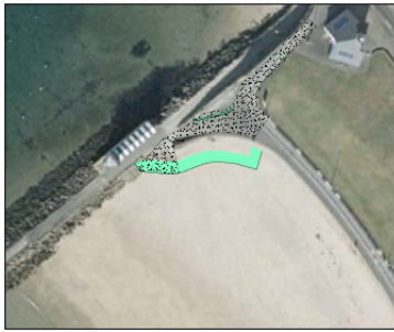
South Pier Access Point Widening of the South Pier Vehicular Access Ramp 1:100
