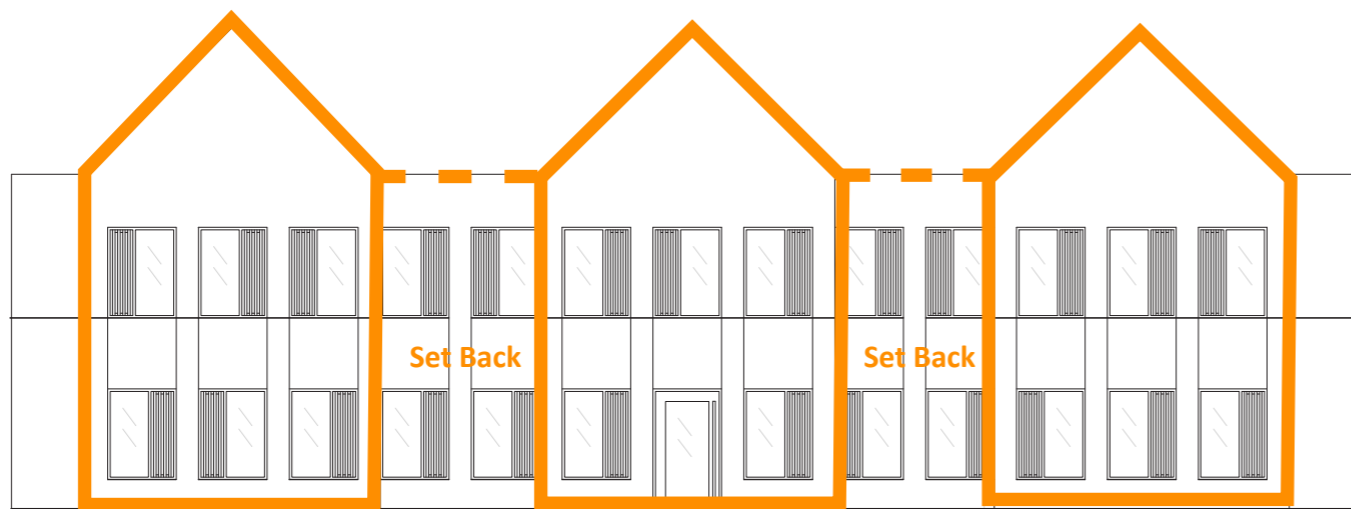
Gable Fronted Elevations with Set Backs - Precedent - Surrounding Properties
