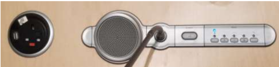
Figure 2: Bosch conference speaker system- Desk Audio Control Unit
